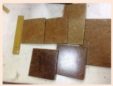
Tiles developed by IIT Researchers using waste including plastic.
